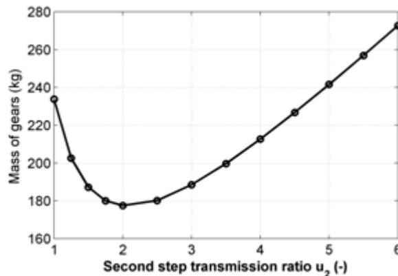
**Figure 1:** Partial ratios versus gear mass of a two-stage helical gearbox Calculation with  $u_h = 10; T_1 = 60000 Nmm; \beta = 12^\circ; k_H = 1.3$
