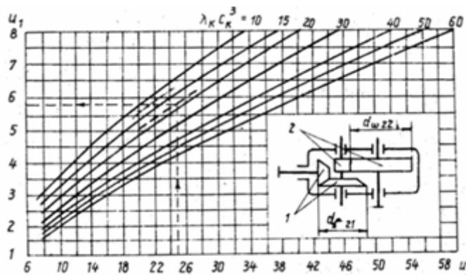
**Figure 2** The gear ratio of the bevel gear set versus the total gearbox ratio [1]
