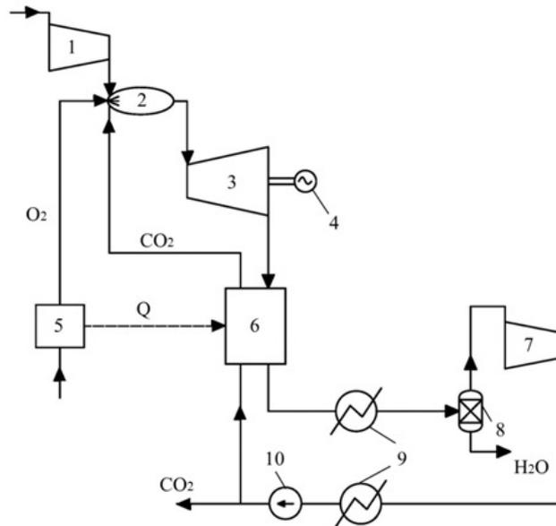
1 – fuel compressor, 2 – combustor, 3 – gas turbine, 4 – power generator, 5 – air split facility, 6 – regenerator, 7 – compressor, 8 – separator, 9 – condenser, 10 – pump
