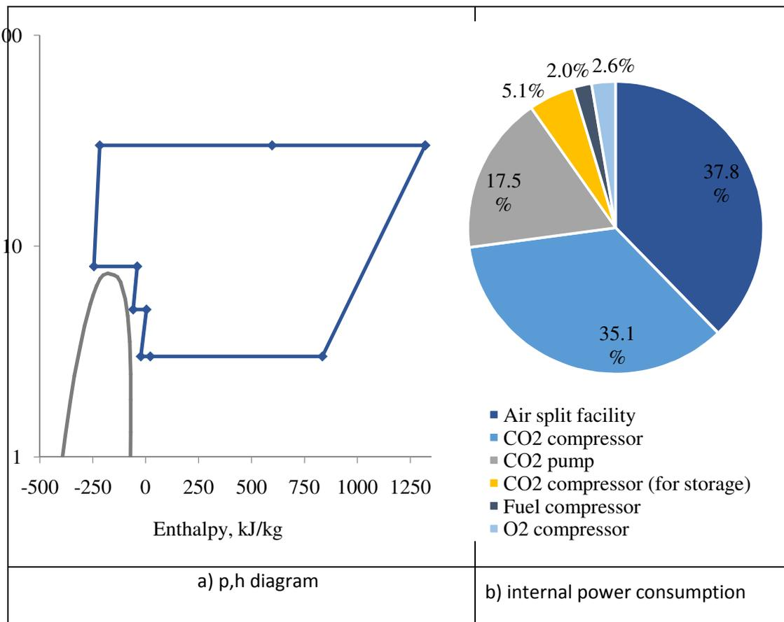
Figure 2 Results of Allam cycle simulation with Excel and REFPROP codes
