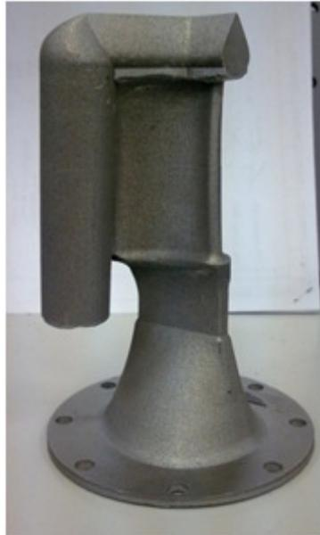
**Figure 2** Prototype blades made by SLM-technology for testing in a liquid-metal thermostat
