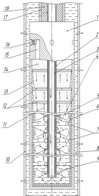
**Figure 3** Downhole electrosteam generator-separator
