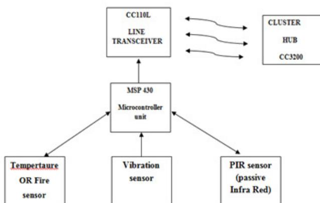
Figure 4 Wireless Transceiver with sensor node
