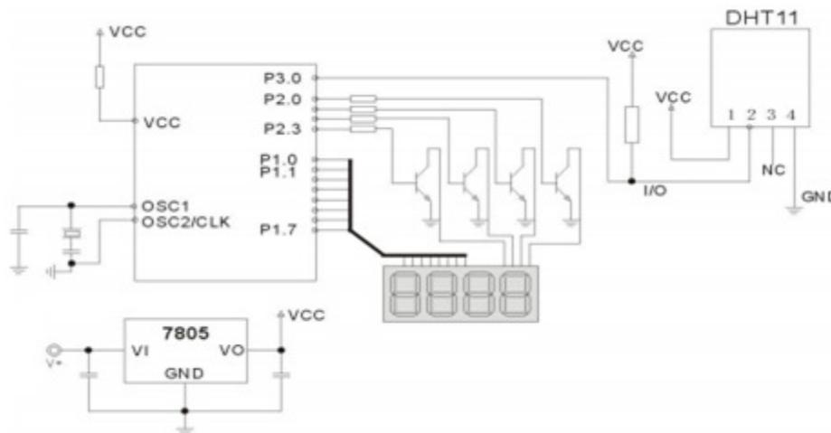
Figure 6 Typical circuit
