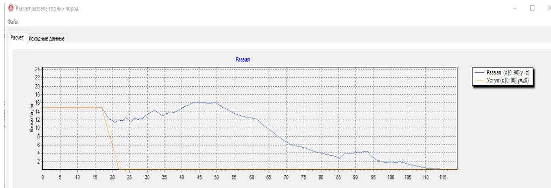
**Figure 5** The shotpile contour of the blasted rock mass constructed using the RazvalPlus automated system.
