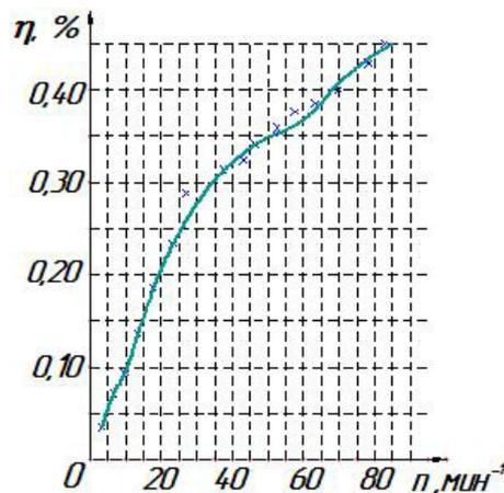
**Figure 6** Dependence of seed crushing ratio on the frequency of rotation of the sowing disc
