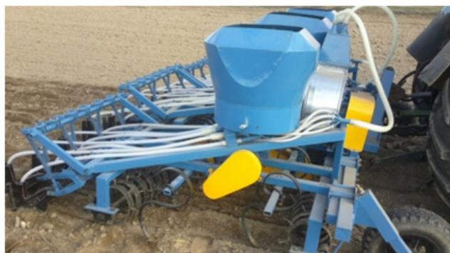
**Figure 3** Carrying out the field testing of a disc pneumatic seed drill
