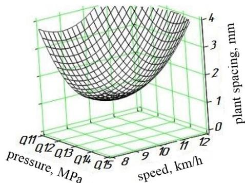
**Figure 7** Dependence of plant spacing (distance between seeds in a row) from pressure and speed of movement
