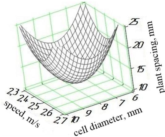
**Figure 5** Dependence of the plant spacing (distance between the seeds in a row) on the belt speed and the diameter of the cells at a disc rotation frequency of  $65 \text{ min}^{-1}$
