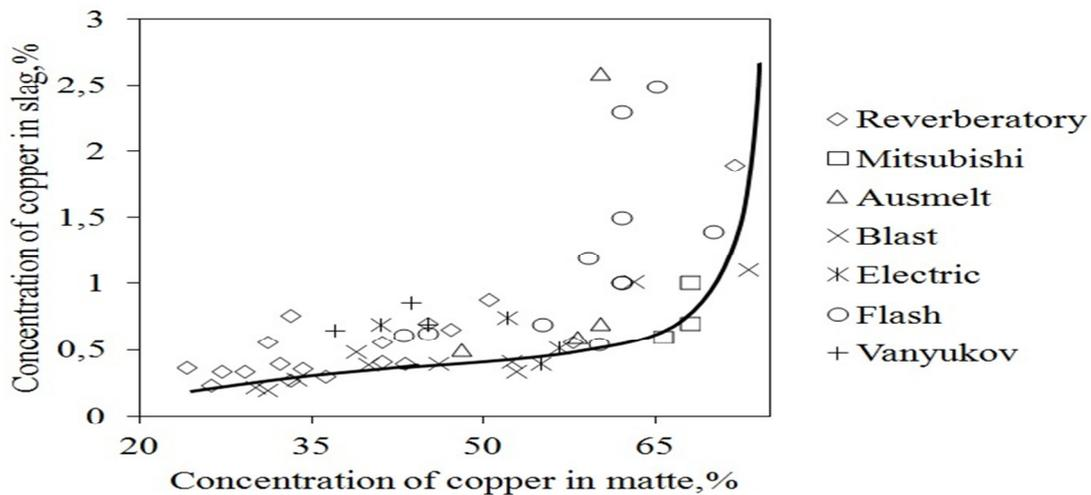
**Figure 1** Copper distribution between slag and matte (solid line characterizes the equilibrium distribution)
