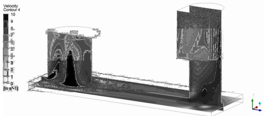
**Figure 2** The nature of the gas-dynamic flow in the flash smelting furnaces
