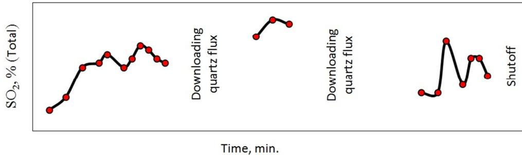
**Figure 4** Experimental measurements of the sulfur dioxide content in the gas phase.
