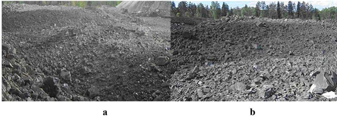
**Figure 2** Rock mass chattering (a - with the use of LGDT, b - with the use of standard charging scheme)
