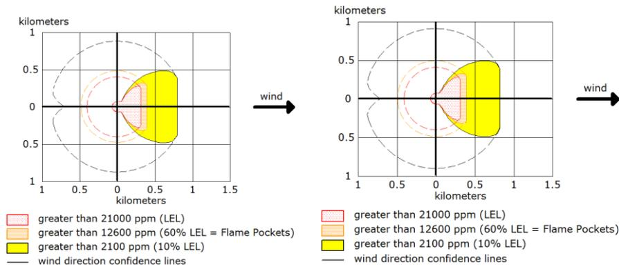
**Figure 5** Bullet Flammable Threat Zone **Figure 6** Tanker Flammable Threat Zone
