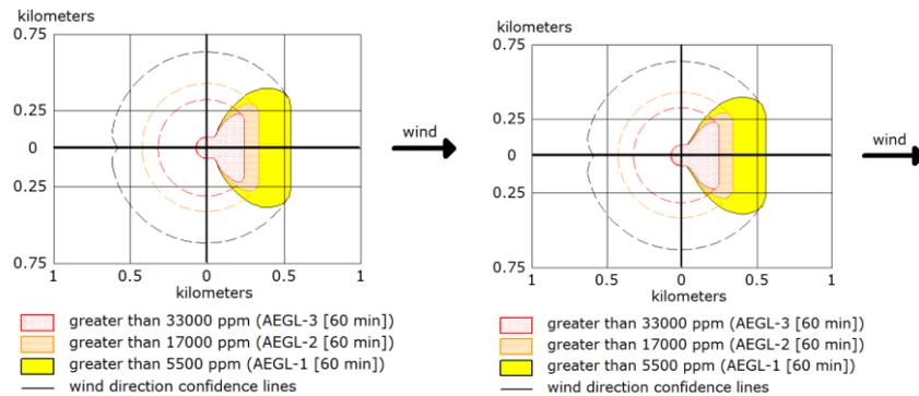
**Figure 7** Bullet Toxic area of Vapour cloud **Figure-8:** Tanker Toxic area of Vapour Cloud
