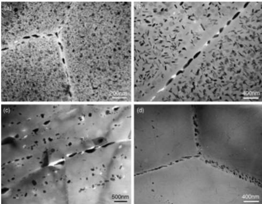
**Figure 4.** Precipitate microstructures in: (a) base metal, (b) HAZ, (c) TMAZ near HAZ, and (d) TMAZ near nugget zone (FSW 7050Al-T651, tool rotation rate: 350 rpm, traverse speed: 15 mm/min) [19].
