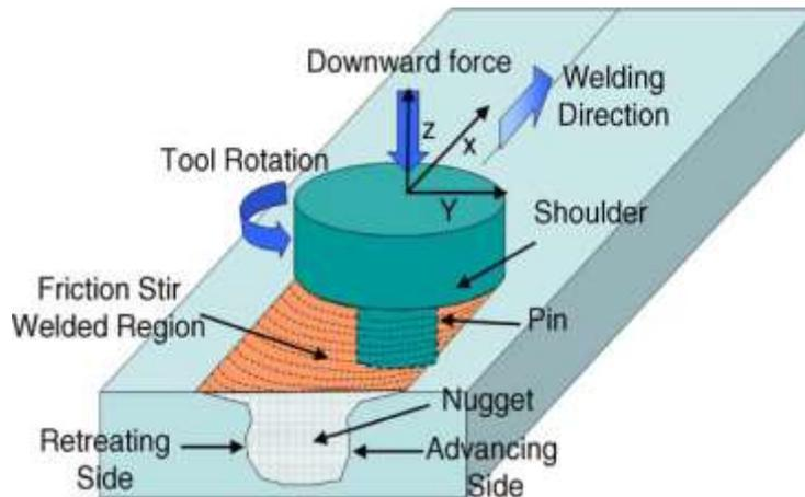
**Figure 1:** Schematic illustration of FSW [28]
