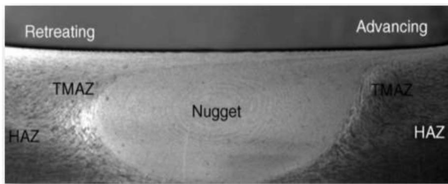
**Figure 2.** Various microstructural zones in FSW [28]
