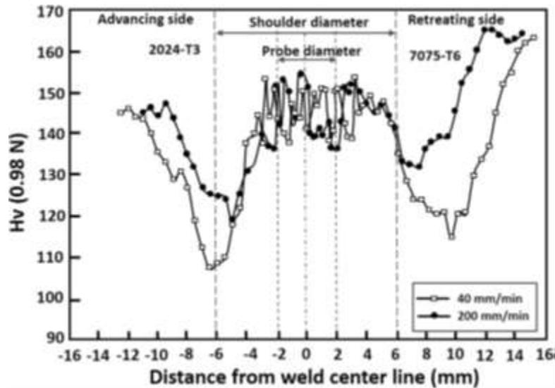
Figure 6 Micro-hardness details of AA2024/AA7075. [24]
