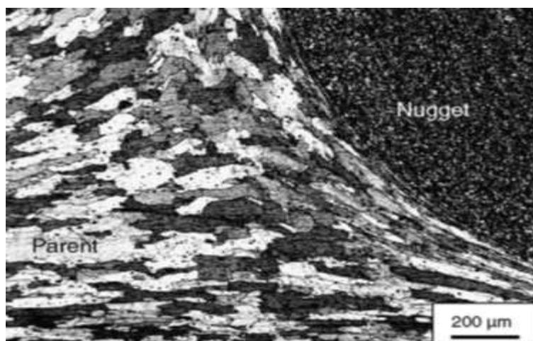
**Figure 3.** Microstructure of thermo-mechanically affected zone in FSP [16].
