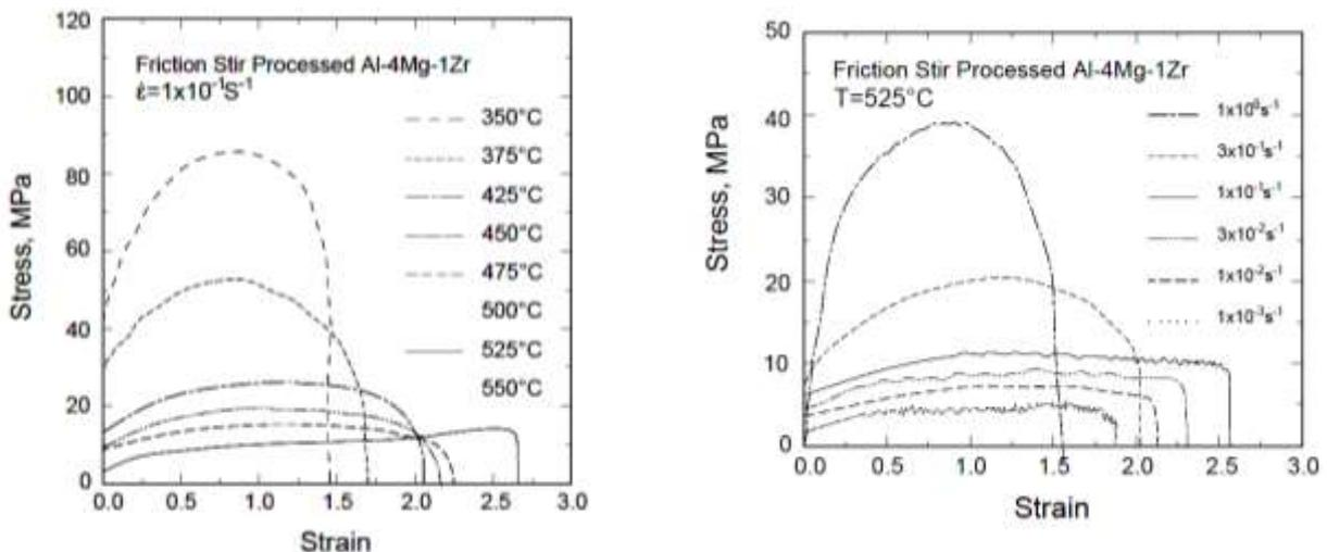
Figure 7. Stress strain properties of friction stir processing Al-4Mg-1Zr, (a) initial strain rate at  $525^{\circ}\text{C}$ , (b) temperature at an initial strain rate  $1 \times 10^{-1} \text{s}^{-1}$  [27]
