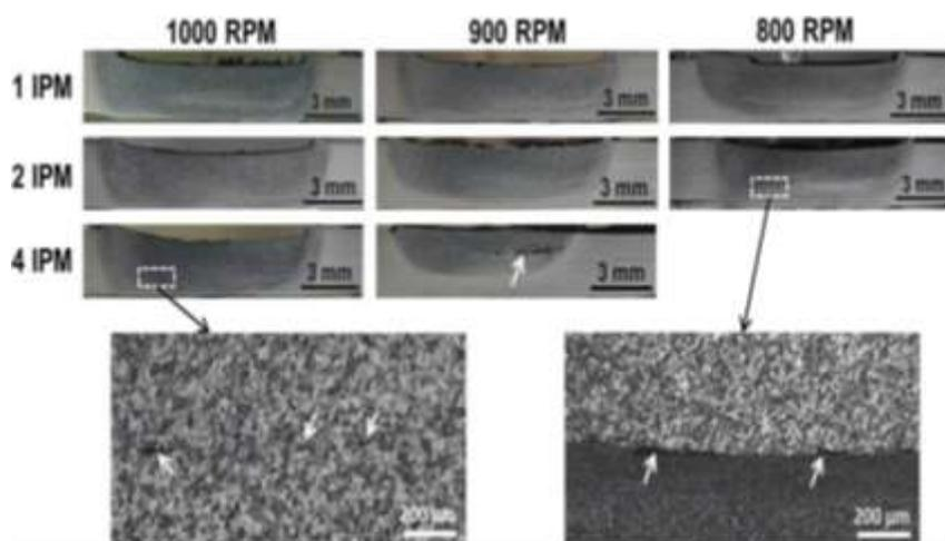
**Figure 5.** Micrographs of contrasting combinations of tool turning speed (RPM) and tool traverse speed (IPM). Note that white arrows shows the processing defects [8]
