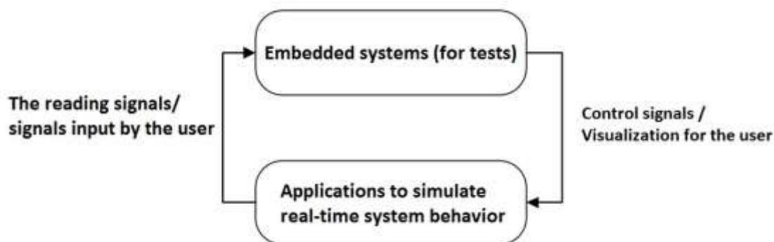
**Figure 3.** Main concept of HIL simulation
