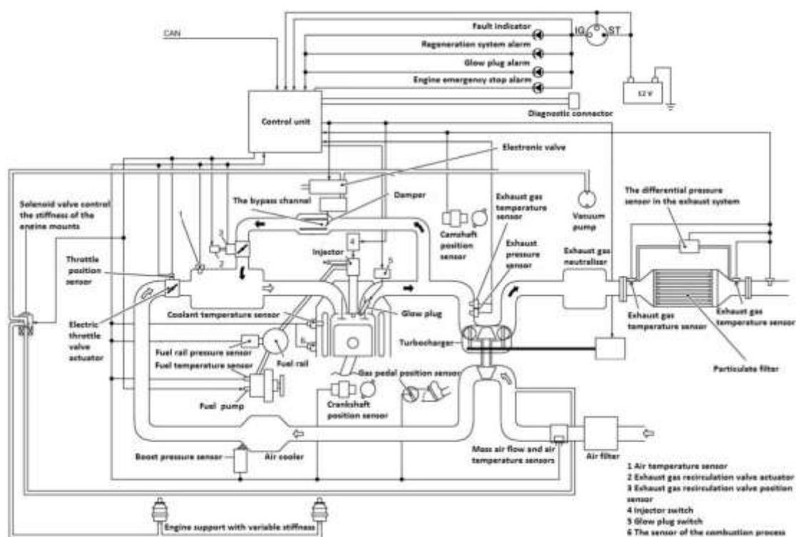
Figure 2. Control system of Russian advanced diesel engine
