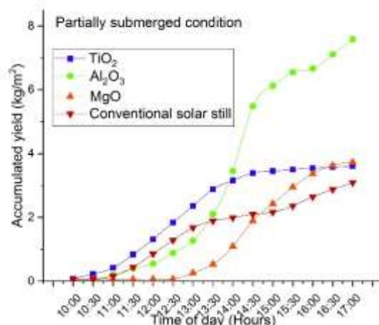
**Figure 5** Variations in accumulated yield of Al<sub>2</sub>O<sub>3</sub>, TiO<sub>2</sub> and MgO nano fluids of modified solar still
