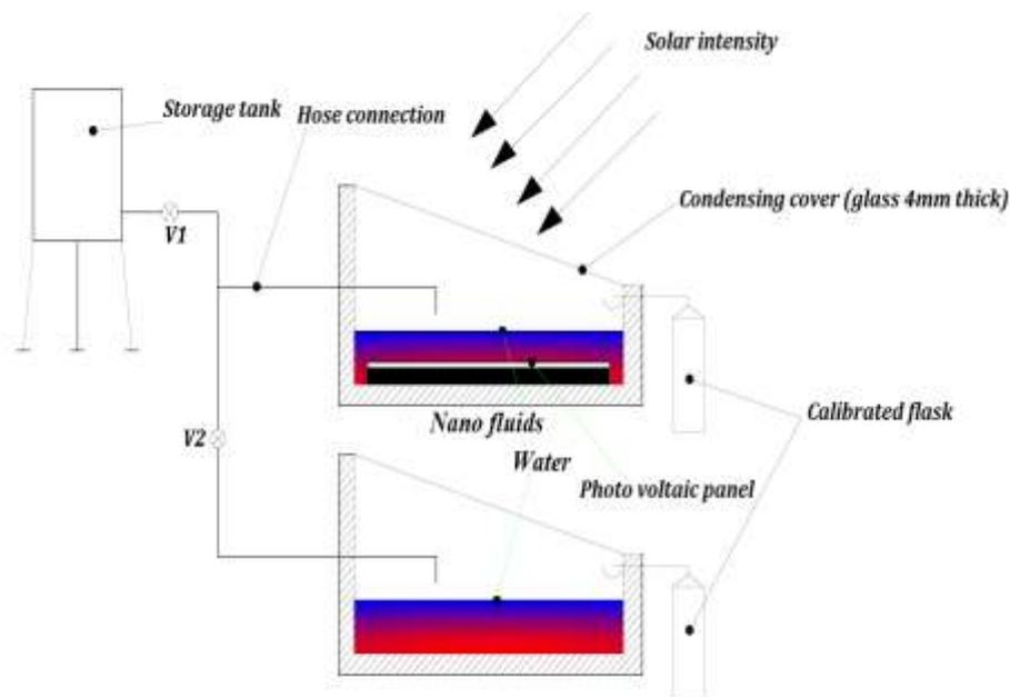
**Figure 1** Schematic diagram of hybrid and conventional solar still
