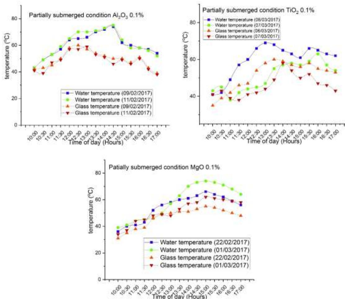
**Figure 4** Variations in water and glass temperature of modified solar still with Al<sub>2</sub>O<sub>3</sub>, TiO<sub>2</sub> and MgO nano fluids
