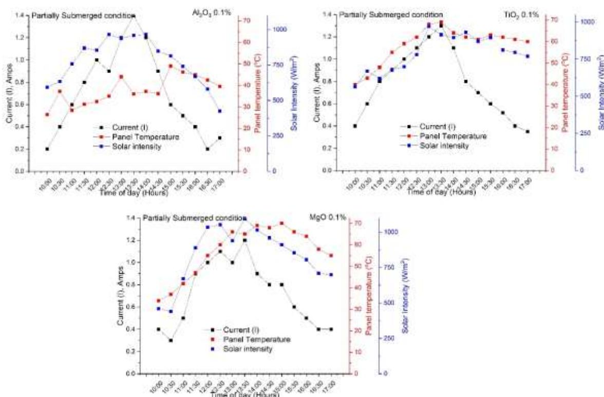
Figure 3 Diurnal variations in panel temperature, current and solar intensity of modified solar still
