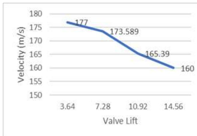
**Figure 13.** Max Air Flow Velocity at 2000 RPM
