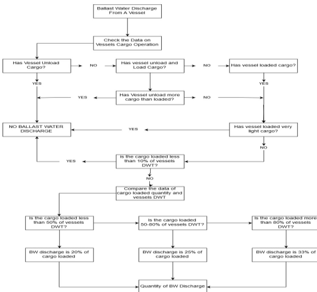
Figure 2 Ballast Water Discharge Assessment Model [3]
