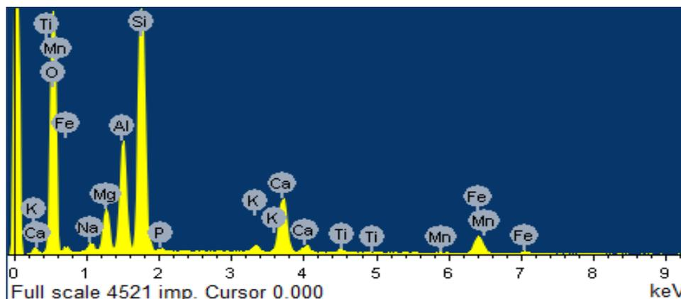
**Figure 1** Scanning electronic microscopy of the basalt sample (the qualitative composition)
