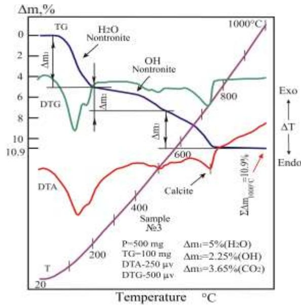
Figure 2 A derivatogram of the Daubaba deposit basalt sample
