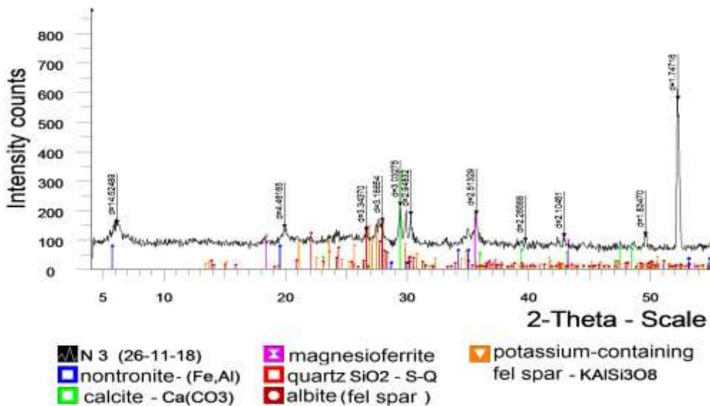
Figure 3 The X-ray phase analysis of the Daubaba deposit basalt sample
