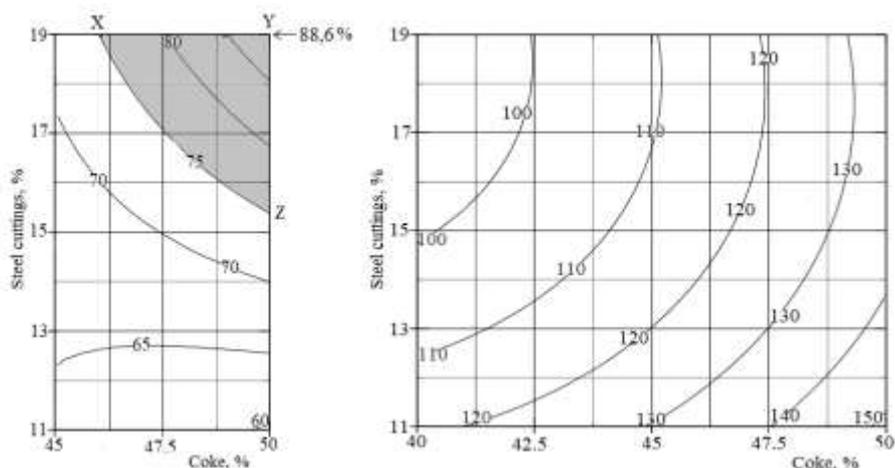
**Figure 6** Effect of the coke and steel cuttings quantity on  $\alpha_{Al(I)}$ , L(II)
