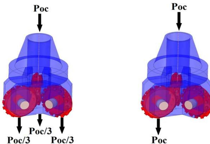
*a* – the load is distributed evenly onto three cutters
