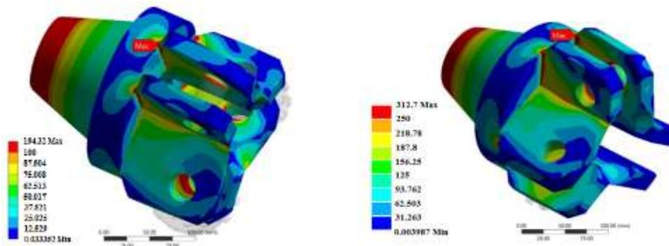
*a* – the load is distributed onto three gear-disc cutters
