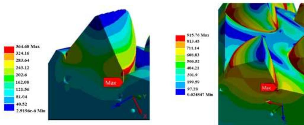
*a* – the load is distributed into three gear-disc cutters evenly
