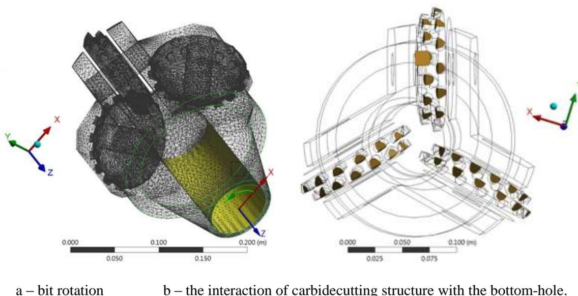
**Figure 3** Boundary loading conditions
