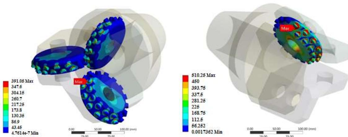
*a*–the load is distributed evenly onto three gear-disc cutters      *b*–the load falls on one gear-disc cutter.
