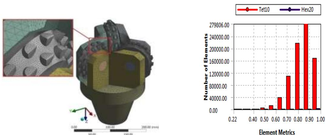
*a* – general view of the finite element model of the bit    *b* – diagram of the quality of elements.
