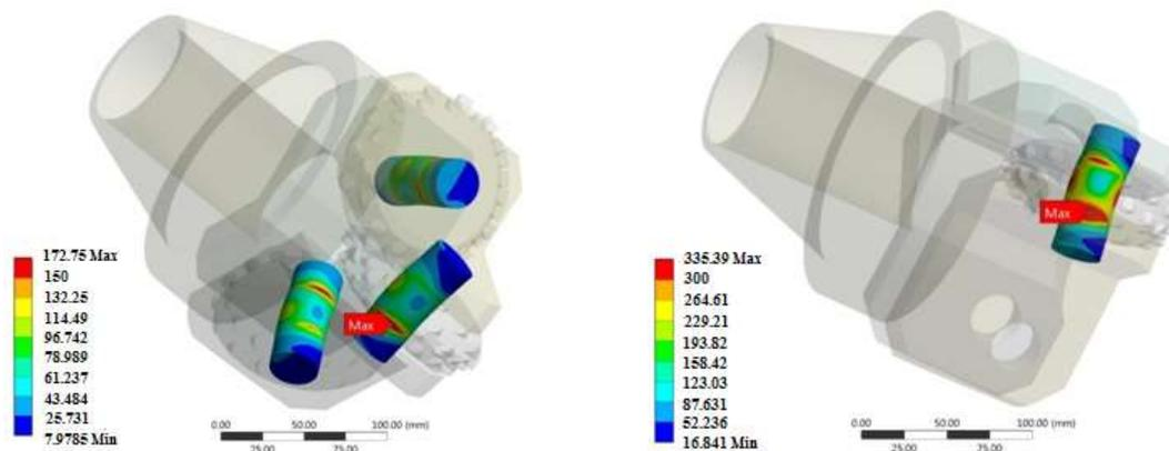
*a* – the load is distributed onto three axes of rotation      *b* – the load falls on one axis of rotation.
