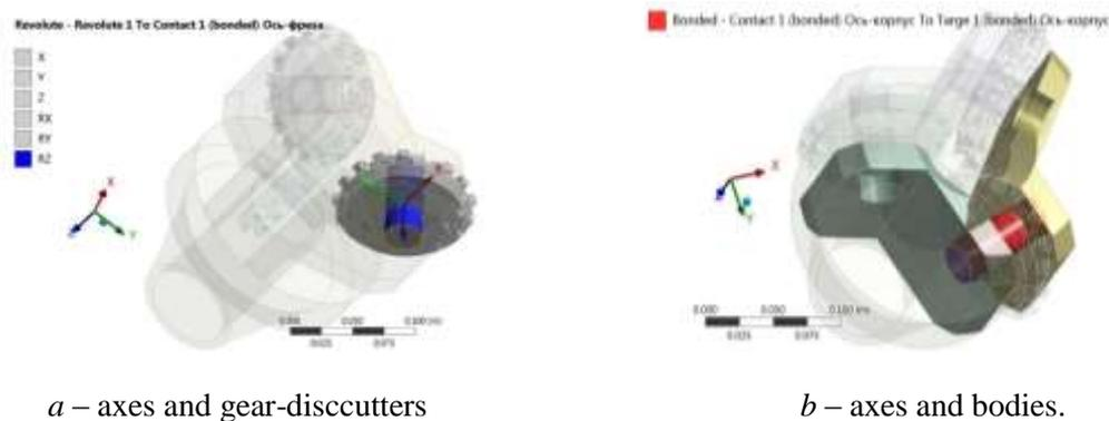
**Figure 2** Model of interfacing elements of the bit
