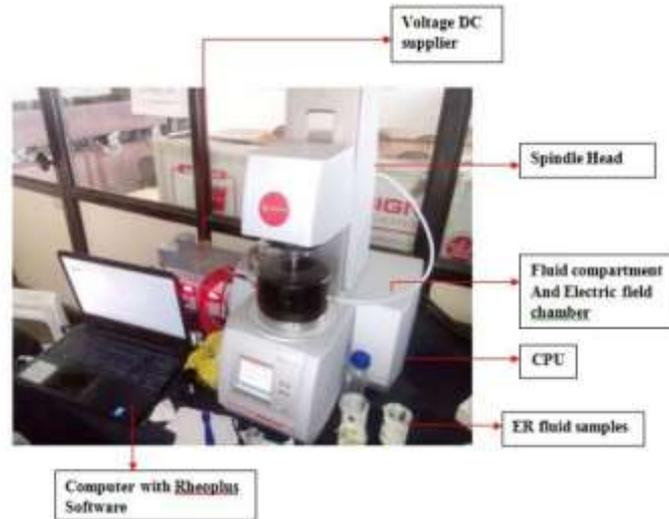
**Figure 7** The experimental set-up with MCR-52
