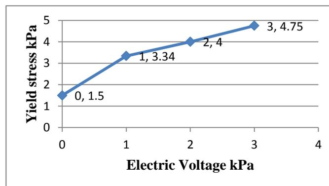
**Figure 8** Dynamic yield strength (kPa) vs. applied electric voltage (kV/mm)
