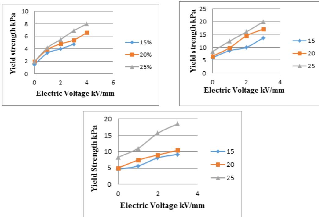
**Figure 9** Yield stress (kPa) vs. electric Voltage (kV/mm) for ER fluid samples with concentration 15%, 20% and 25% of (a) Bare BTO (b) Urea coated BTO (c) Acrylamide coated BTO
