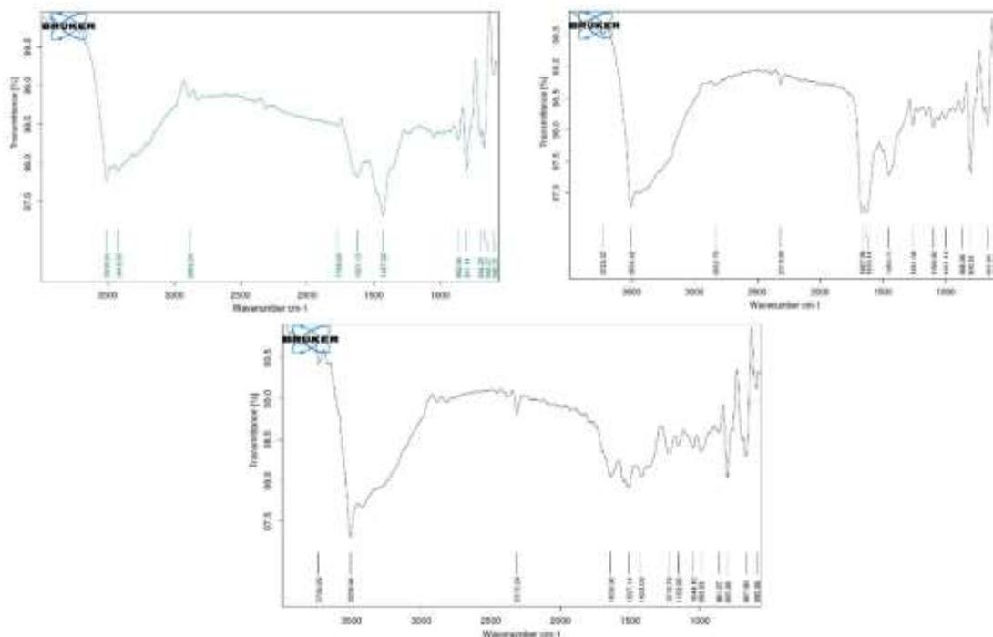
**Figure 4** (a) FT-IR of bare BTO powder (b) FT-IR of Urea coated BTO powder (c) FT-IR of Acrylamide coated BTO powder
