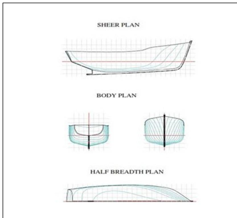
**Figure 2.** Redrawing of Batang Type Traditional Fishing Boat
