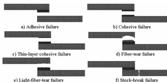
**Figure.5:** Types of Failure modes of Laminate
