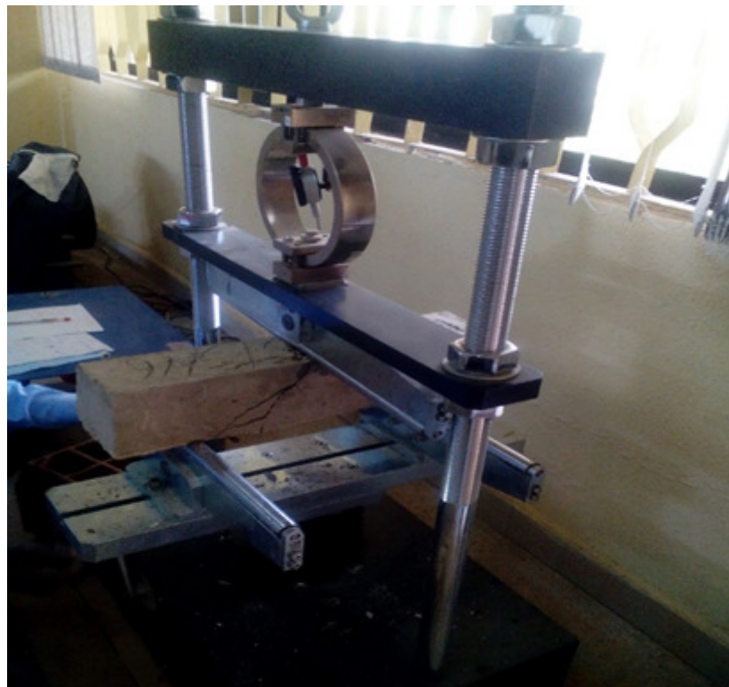
Plate 1 Flexural machine and flexural beam under load
