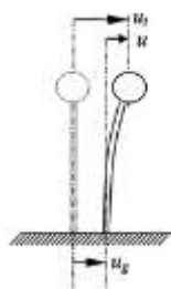
Figure 1 Earthquake induced motion of an SDOF system[5][9]
