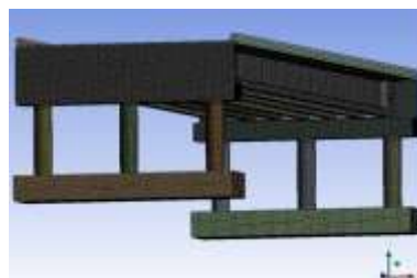
Figure 4 3D solid element of bridge model
