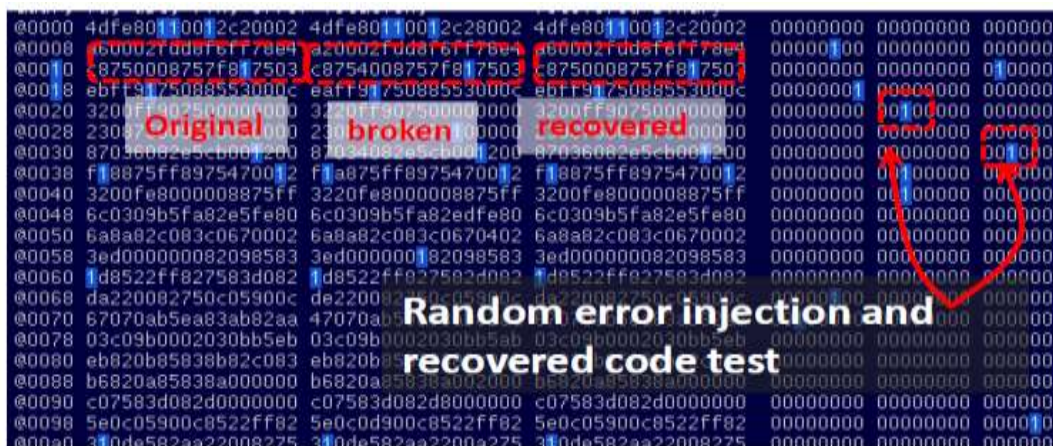
Figure 8 Random bit error injection caused by human-activity and recovered binary pattern by using the proposed approach
