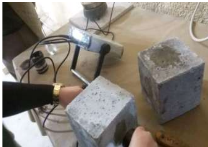
Figure 1 Ultrasonic pulse velocity (UPV) test
