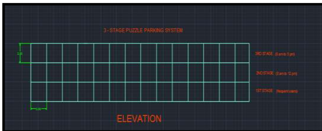
Figure 7 Elevation of 3 Stage Puzzle Parking System
