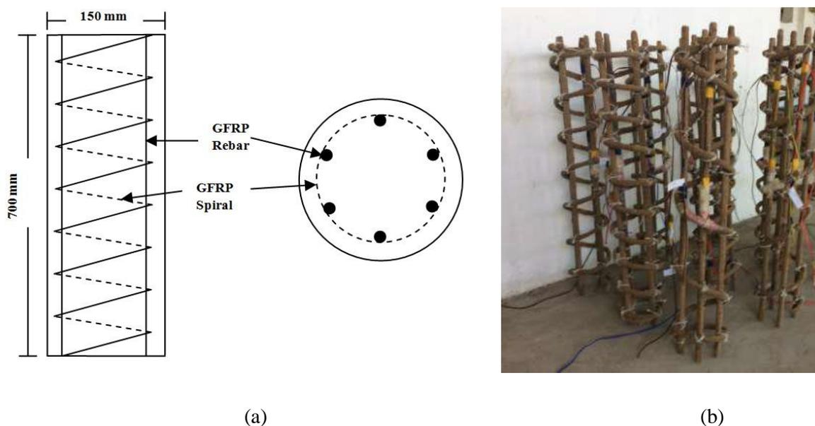
**Figure 1** Glass Fiber Reinforcements used in short columns
