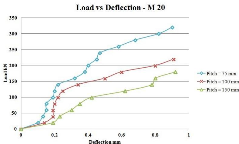
**Figure 3** Load vs Deflection graph of M 20 grade column specimens
