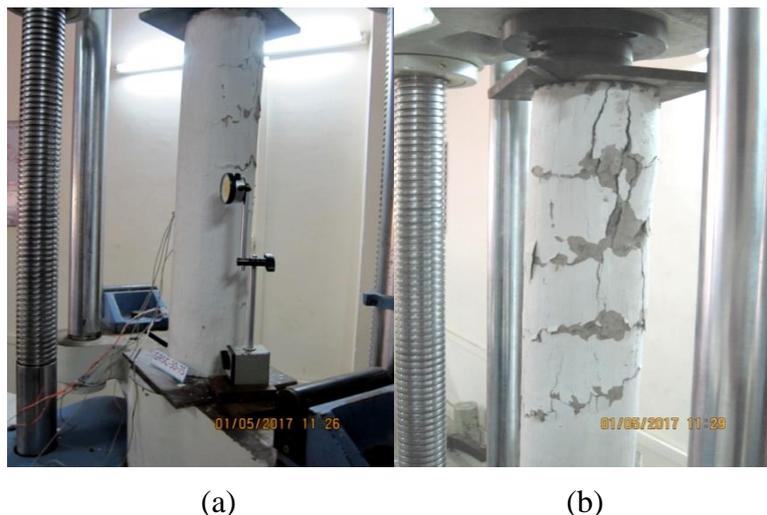
**Figure 2** GFRP Columns tested in UTM
