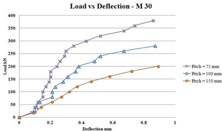
**Figure 4** Load vs Deflection graph of M 30 grade column specimens
