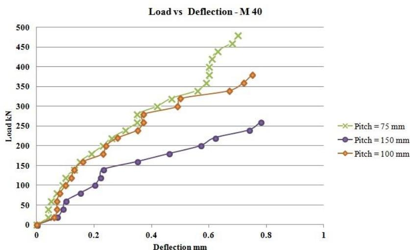
**Figure 5** Load vs Deflection graph of M 40 grade column specimens
