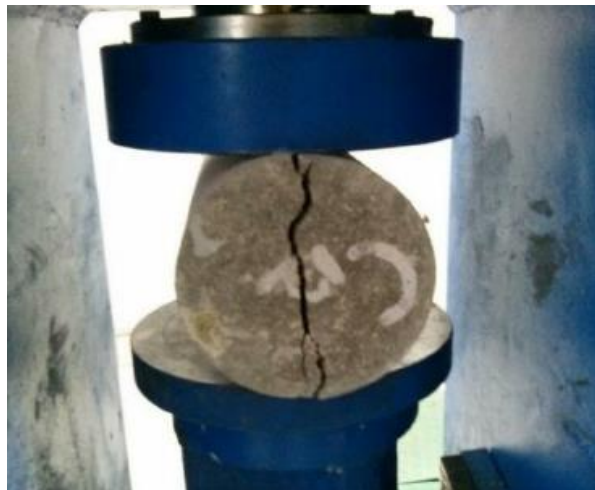
Figure 3 Split Tensile Strength test Setup
