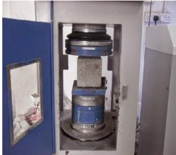
Figure 2 Compressive Strength Test Setup
