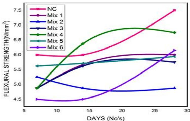
**Figure 8** Result of Trialanalysis showing the flexural strength of concrete with different proportion replacement of textile sludge.
