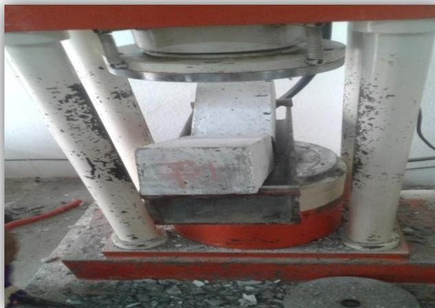
**Figure 7** Testing Image on Flexural Strength
