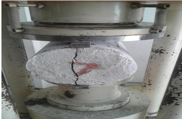
**Figure 5** Testing image on split tensile strength
