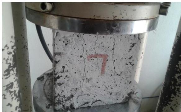
**Figure 3** Testing on Compressive Strength
