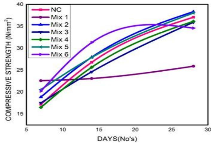
**Figure 4** Result of Experimental investigations showing the compressive strength of concrete with different percentage replacement of textile sludge.
