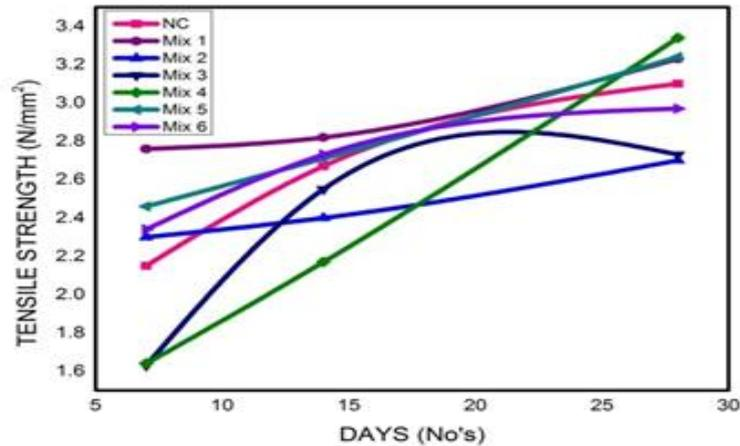
**Figure 6** Result of Experimental investigation showing the split tensile strength of concrete with different percentage replacement of textile sludge.
