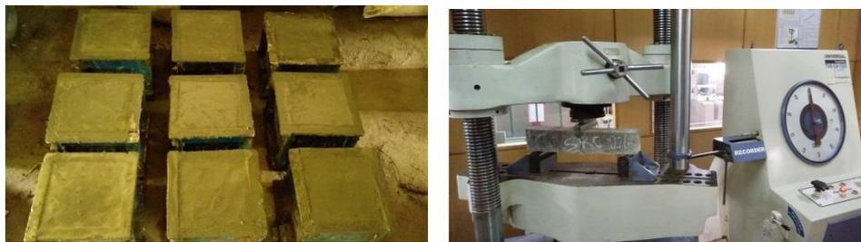
Figure 1 Casted and tested specimens
