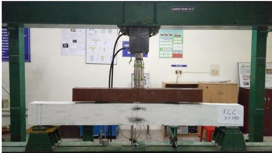
Figure 4 Experimental set-up for the test specimens
