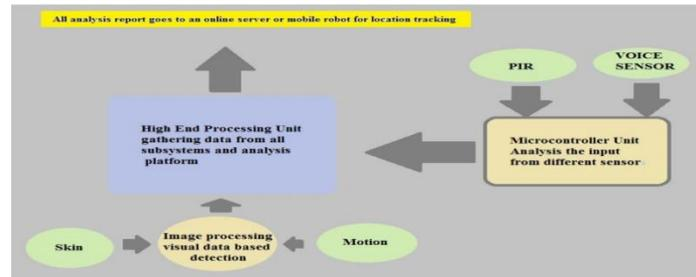
**Figure 1** Block diagram of Complete System
