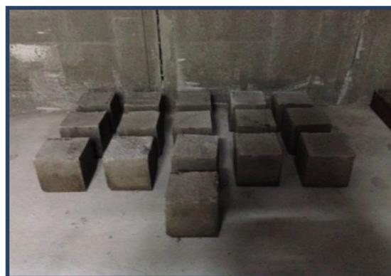
**Figure 3** Pouring of Foam Concrete Cubes in Moulds **Figure 4** Foam Concrete Cubes After Casting
