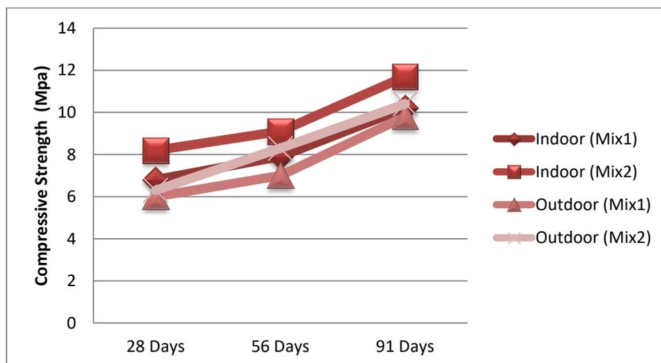
**Figure 8** Strength over time for biomass indoor and outdoor specimens
