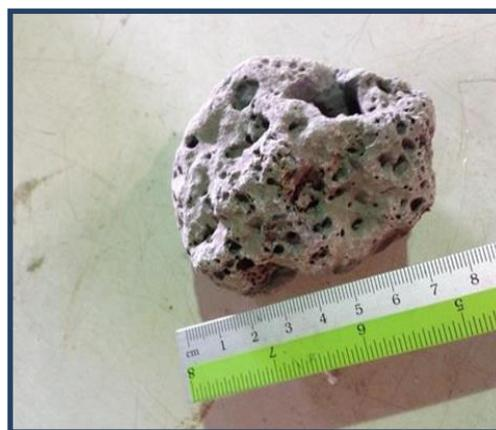
Figure 2. Recycled Biomass Aggregate (RBA)
