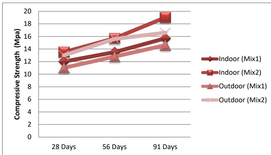
**Figure 7** Strength over time for sand indoor and outdoor specimens
