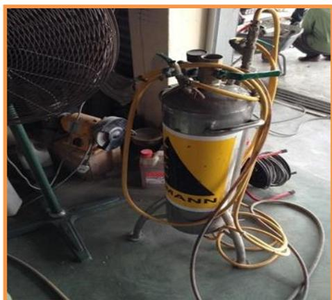
Figure 2. Foaming Generator
