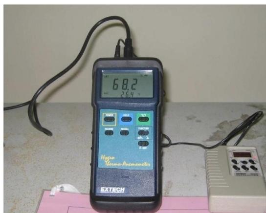
**Figure 6** Electronic humidity sensor and thermometer
