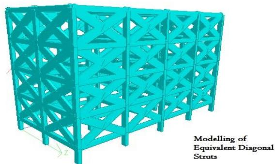
**Figure 5** Modelling of compression strut
