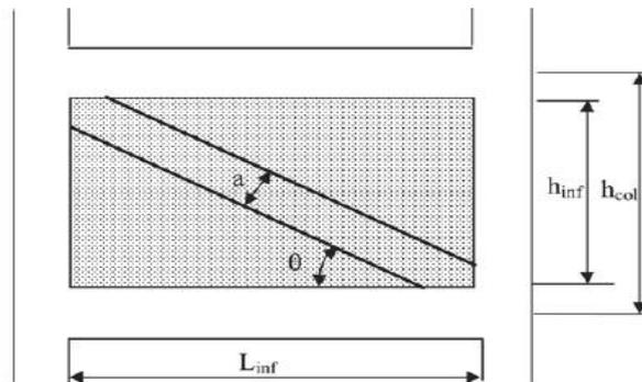
1. Equivalent diagonal compression strut model for infill walls.
