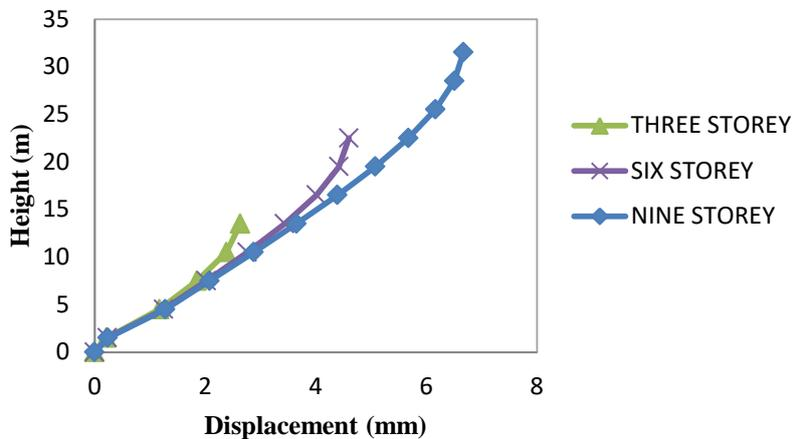
Figure 8 Displacement for without infill models
