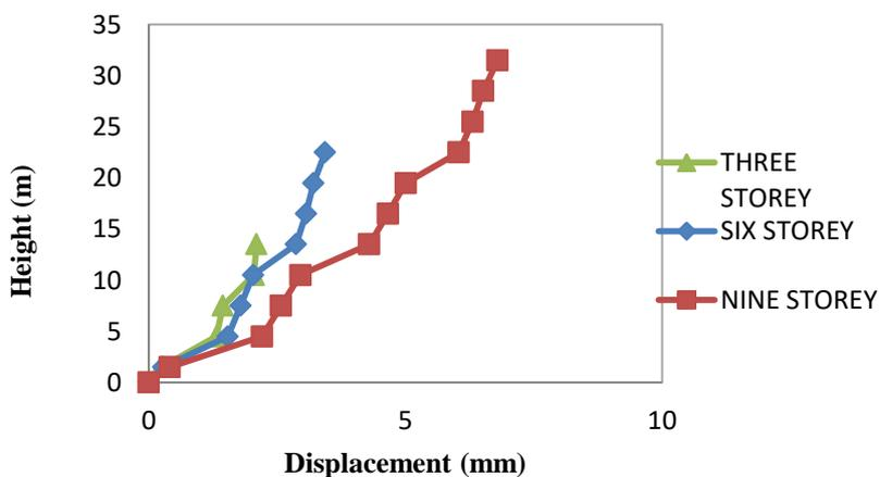
Figure 10 Displacement for Partial infill models
