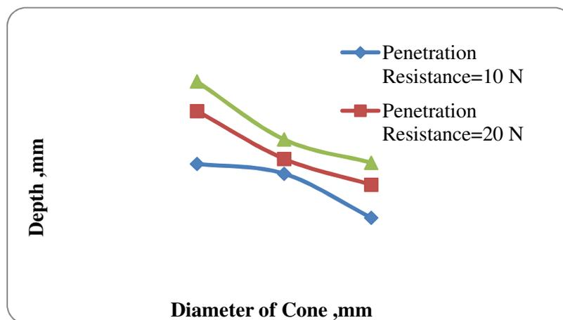
**Figure 5** Depth of penetration vs Cone Diameter in different load
