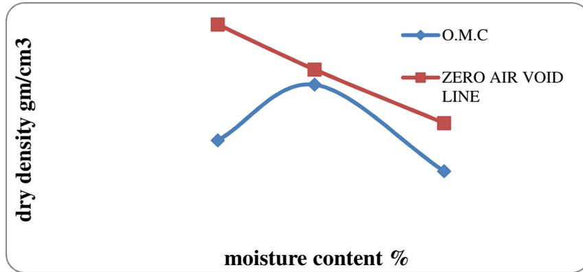
Figure 2 Compaction characteristics of sand
