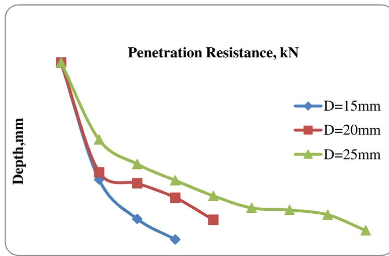
**Figure 4** Penetration resistance vs Depth in mm with different diameter of cone
