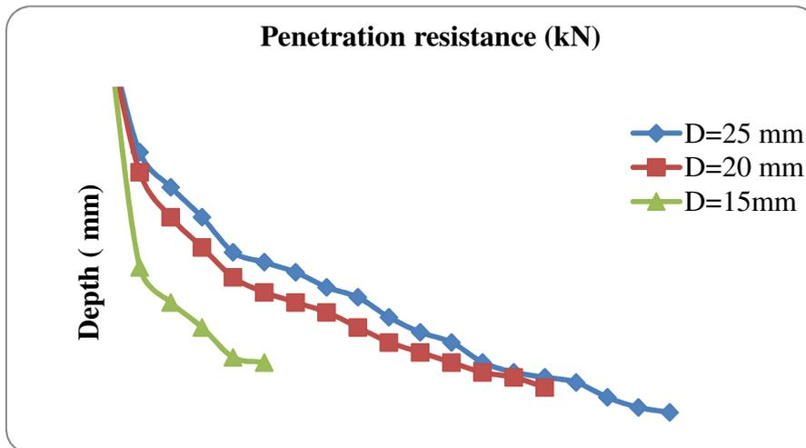
**Figure 7** Penetration resistance vs Depth with different diameter of cone
