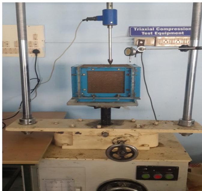
Figure 3 Setup of Cone Penetration Test on sand
