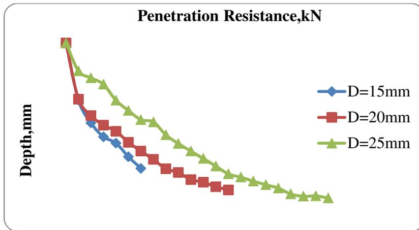
**Figure 6** Penetration resistance vs Depth with different diameter of cone in saturated sandy soil
