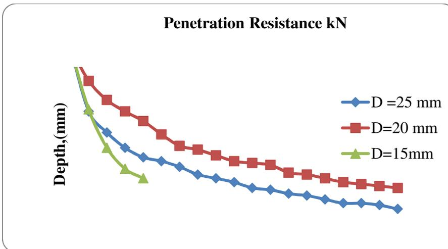
**Figure 8** Penetration resistance vs Depth with different diameter of cone
