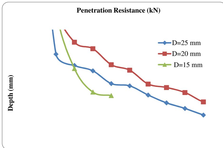
**Figure 10** Penetration resistance vs Depth with different diameter of cone
