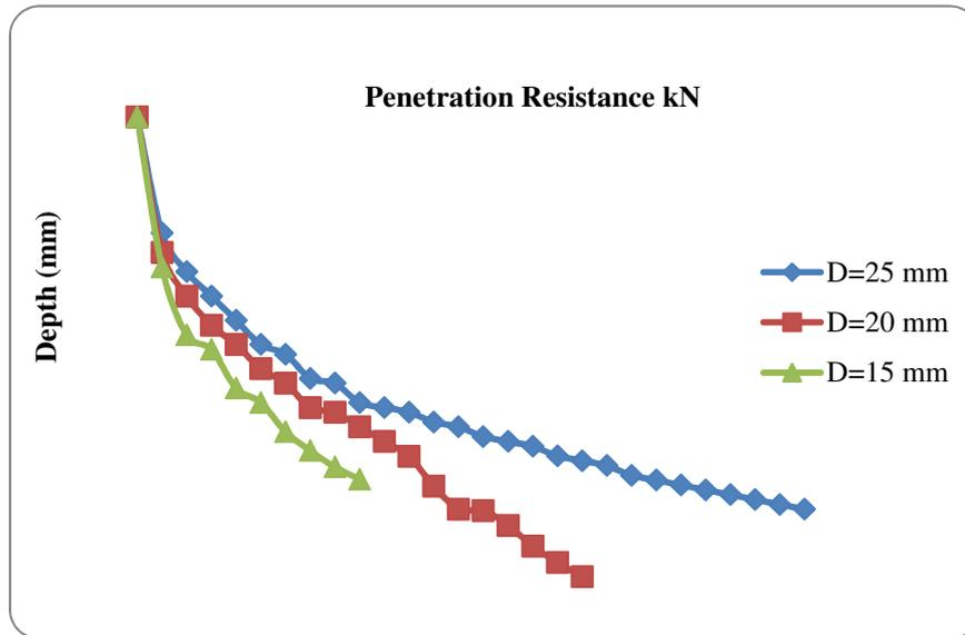
**Figure 9** Penetration resistance vs Depth with different diameter of cone
