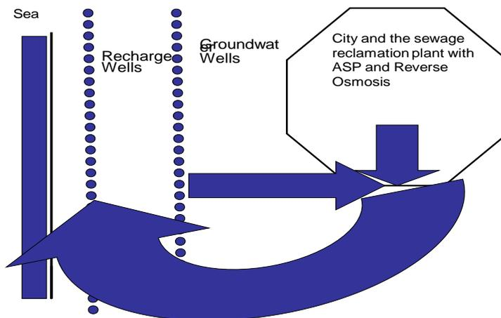
Figure 1 The Schematic of Orange County Advanced Treated Sewage Injection wells along the Pacific coast to achieve (a) seawater intrusion barrier & (b) indirect potable use of sewage
