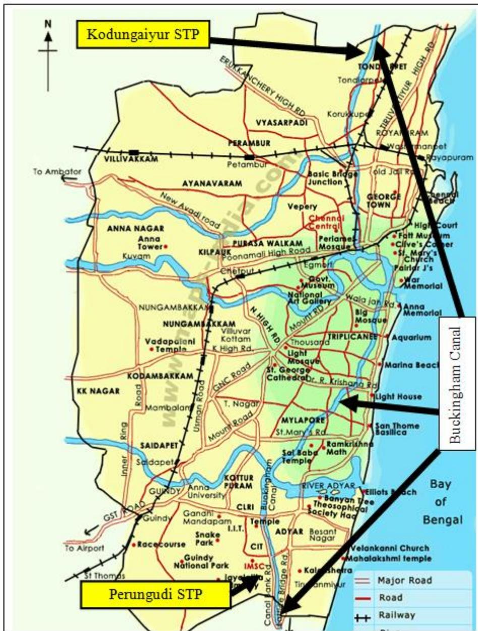
**Figure 2** The Buckingham Canal enters Chennai from the north and exits in the south. It is a waterway and not a river, The 2 STPs are ideally located for a connecting pipeline between the two along the canal bank and for driving injection bore wells along the canal alignment parallel to the coastline and inject the treated sewage.
