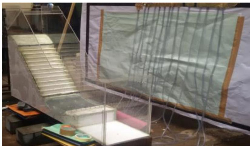
**Figure 2** Experimental setup of ogee profile stepped spillway in laboratory
