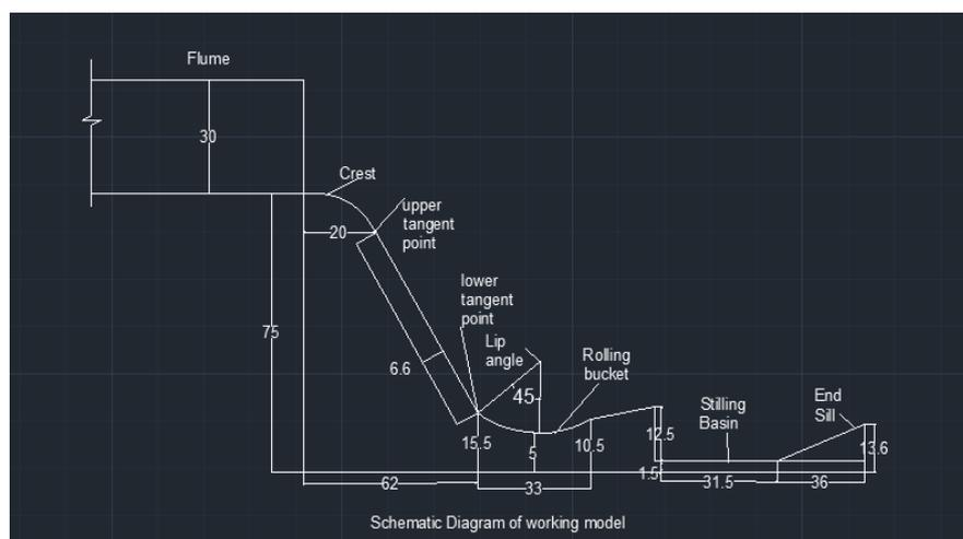
**Figure 1** Typical cross section of an ogee profile spillway model
