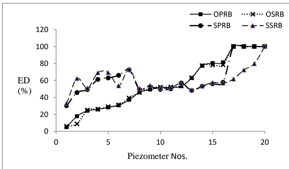
**Figure 5** Graph of Energy Dissipation at 4 m head for all models
