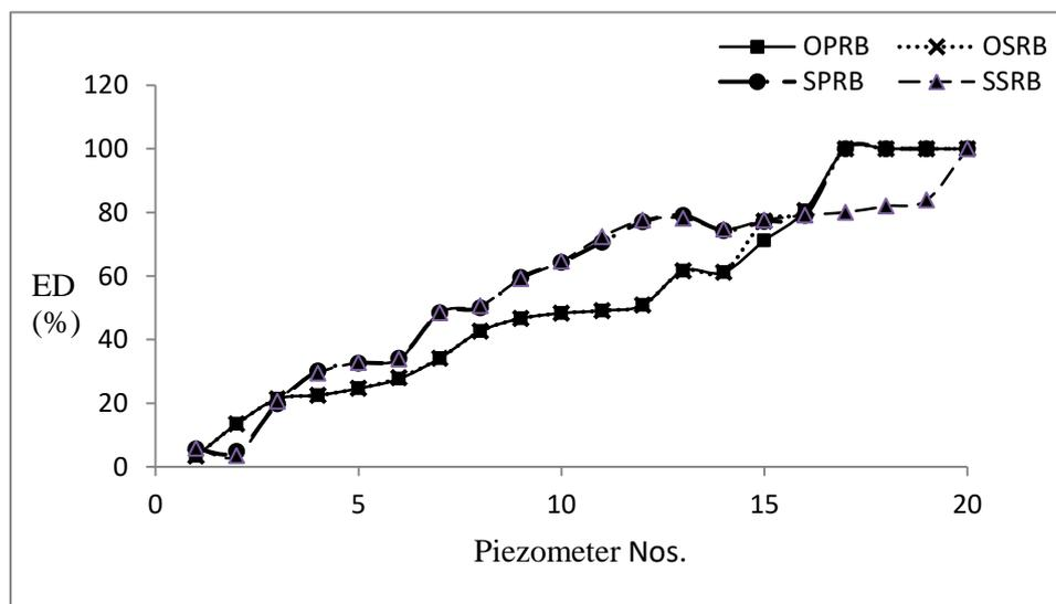
Figure 6 Graph of Energy Dissipation at 6 m head for all models
