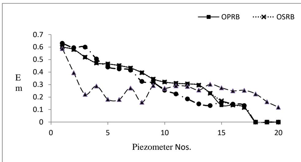
**Figure 4** Graph of specific energy distribution at 6m head for all models
