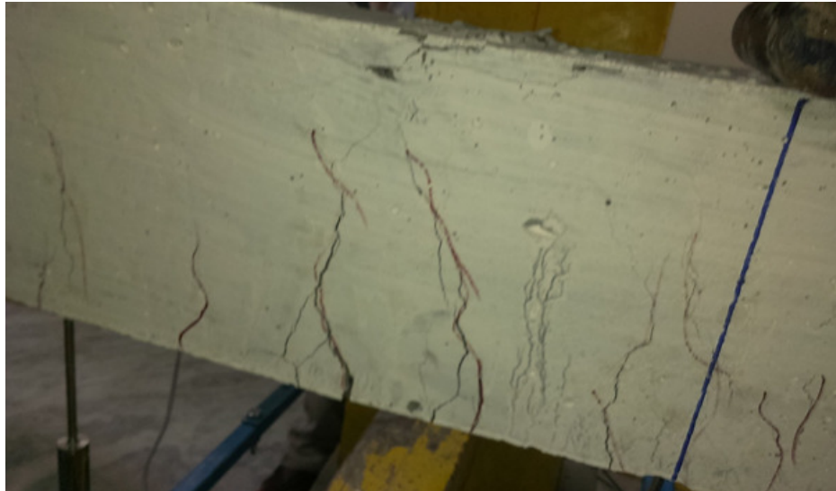
Figure 3.5 Flexure control beam
