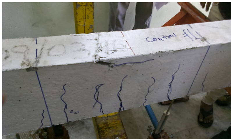
Figure 3.4 Flexure control beam
