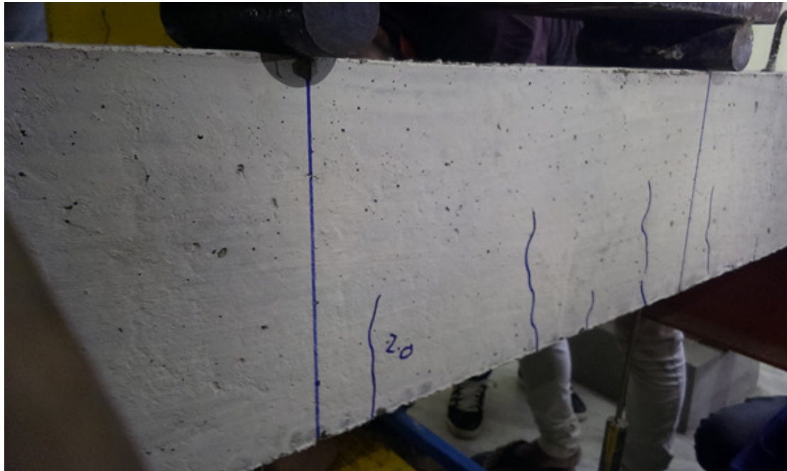
Figure 3.9 70% Preloading Flexural Wrapped Beam
