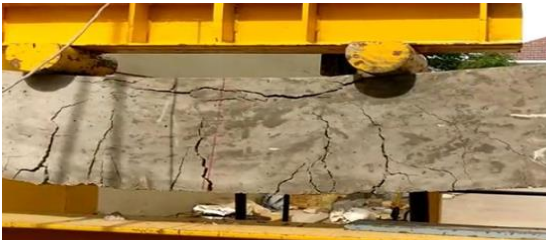
Figure 11 Flexural Strength testing of Beams
