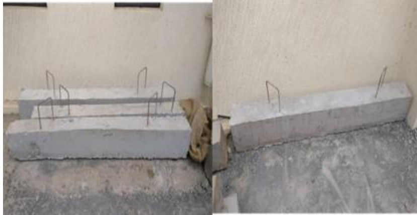
Figure 10 Casted Beam Specimens
