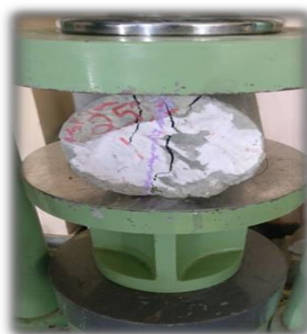
Figure 6 Split Tensile Strength test on Cylinder Specimen
