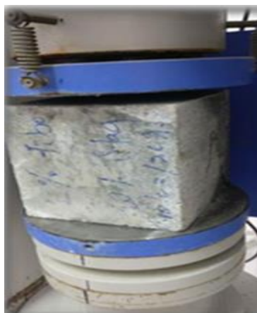
Figure 3 Compression Testing of Cube Specimen
