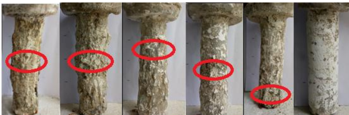
Figure 4 Bulging of Stone column for LS column, SG+LS column, Reinforced LS+SG columns with encasement lengths of D, 2D, 3D and 4D respectively
