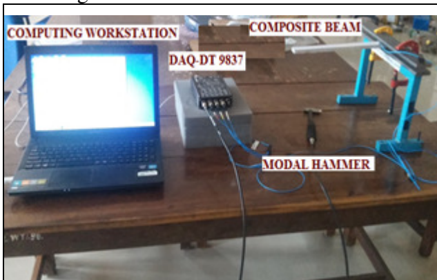
Figure 5 Setup for Experimental Modal Analysis
