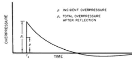
Figure 3.22. Variation of overpressure with time at a point on the surface in the region of regular reflection.
