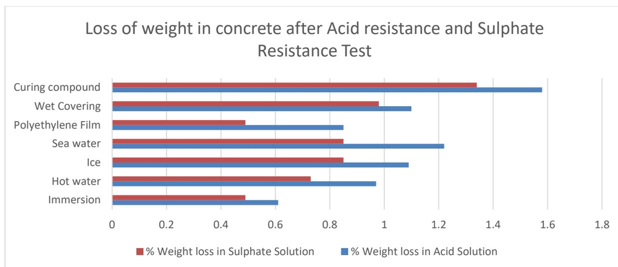
**Figure 1** Loss of weight in concrete after Acid resistance and Sulphate Resistance Test
