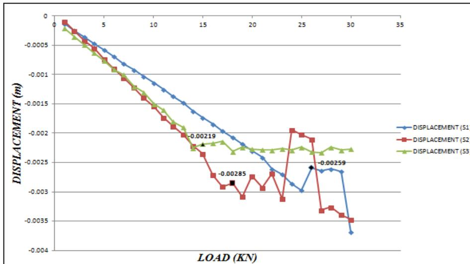
Figure 4 Load vs Displacement curve for all the three connections
