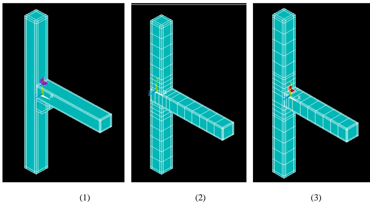
**Figure 1** ANSYS model of precast beam and column connection with corbel (S1). **Figure 2:** ANSYS model of precast beam and column connection with beam-column visible connection (S2). **Figure 3:** ANSYS model of precast beam and column connection hidden connection (S3).
