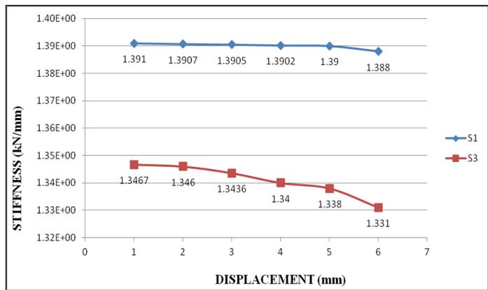
Figure 7 Stiffness vs Displacement graph for structures S1 and S3
