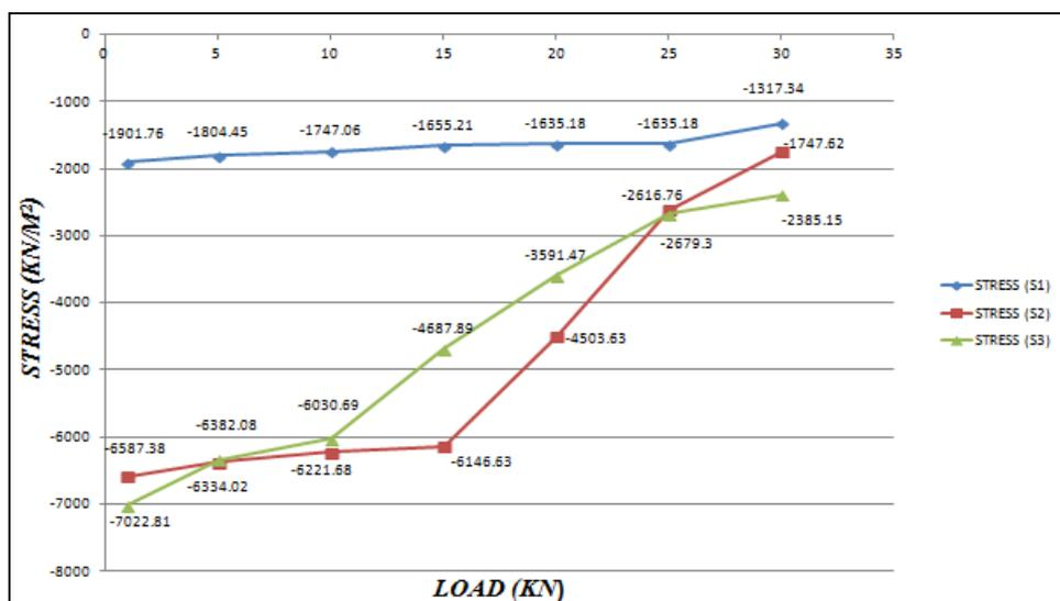
Figure 5 Load vs Stress curve for all the three connection
