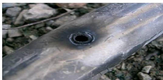
**Figure 6** Cable Fault, 1-Core 11kv XLPE Cable
