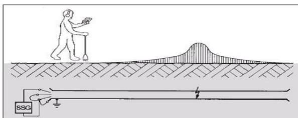
**Figure 5** Schematic Connection and Shape of Acoustic Signal – Acoustic Fault Location
