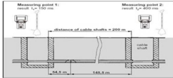
**Figure.7** Manhole Arrangement, Cable Laid In PVC Pipe, Acoustic Signal Only Audible on Manhole Cover
