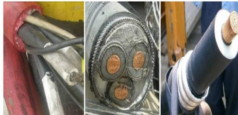
**Figure.2.** 3-core EPR, incl. 3-core XLPE 11kV 1-core XLPE 115kV Data line, radial type
