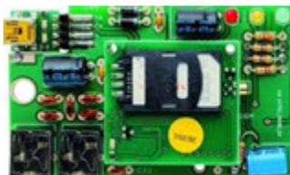
Figure 3 GSM Module
