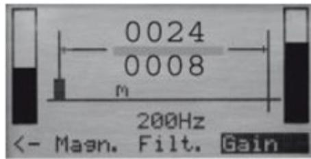
**Figure.7.1** UL30 Display, Manhole Mode, Display of Two Propagation Time Values Used
