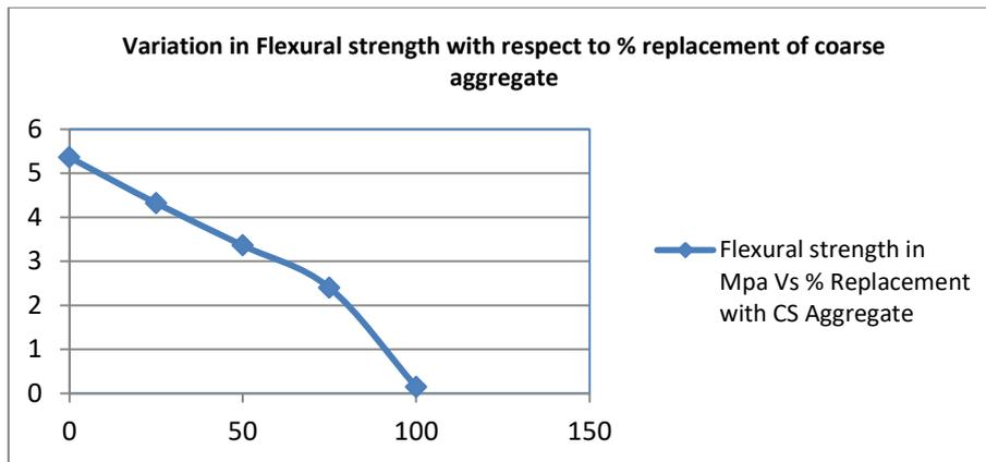
**Figure 8** Variation in Flexural Strength Vs % Replacement of CS Aggregate
