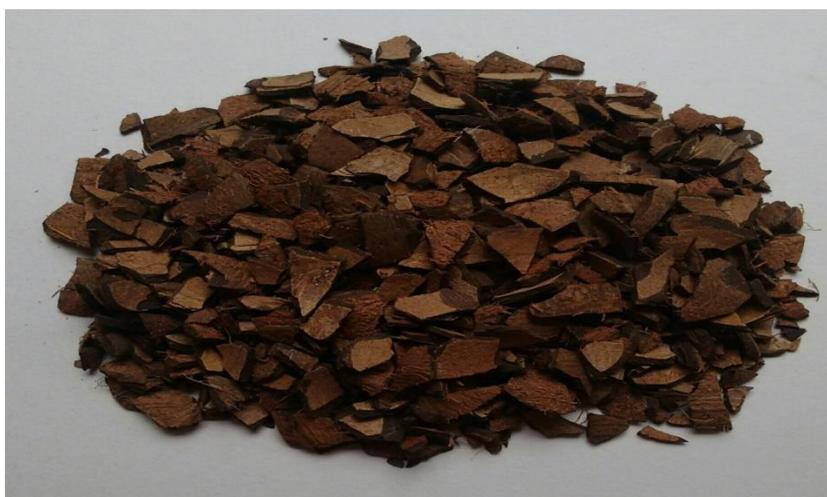
**Figure 2** Coconut Shell Aggregates
