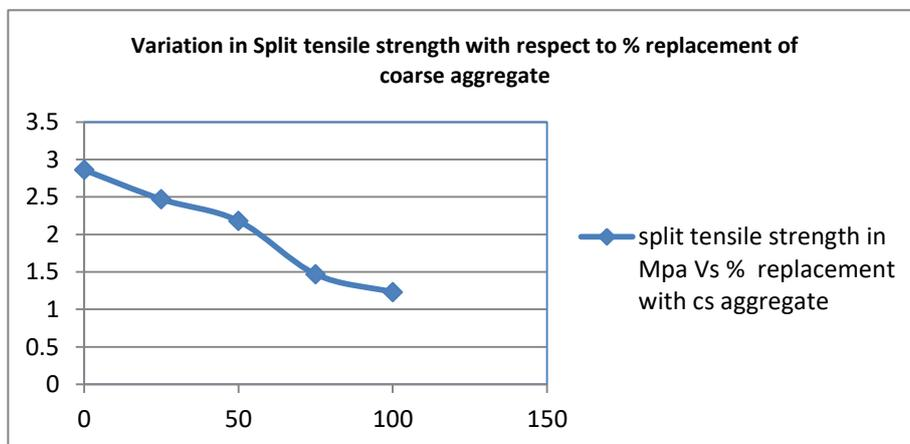
**Figure 6** Split Tensile Strength Vs % Replacement of Coarse Aggregate
