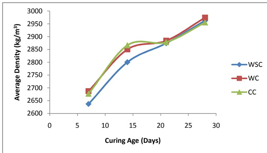
**Figure 5** Average Density at various ages and types of curing
