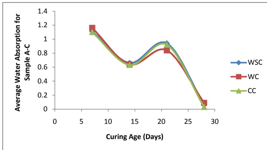
**Figure 3** Average Water Absorption at Different Curing Age (Days)
