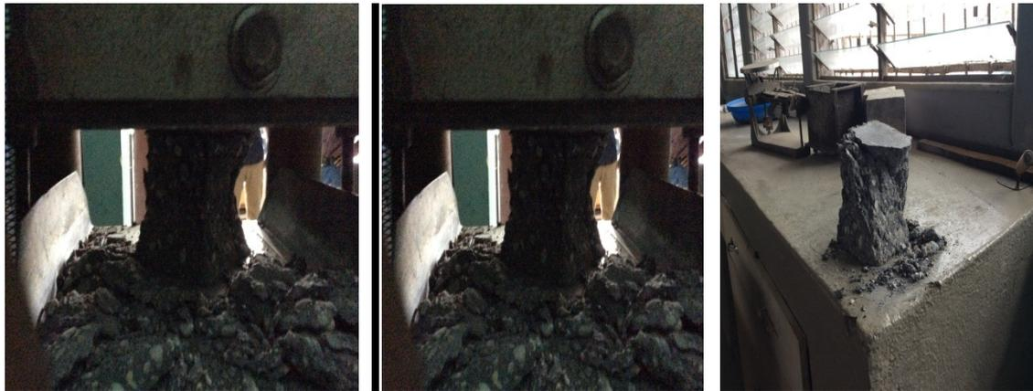
**Figure 4** Plates 3 Failure Characteristics of HSHP under Compressive load
