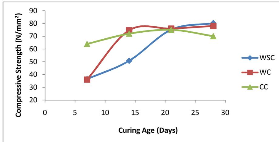
**Figure 3** Variation of Compressive strength various duration and type of curing
