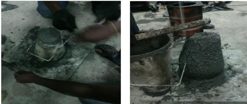
**Figure 2** Plate 2 Slump workability Tests process
