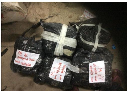
Plate 1 (c) Wet sand curing (WSC)
