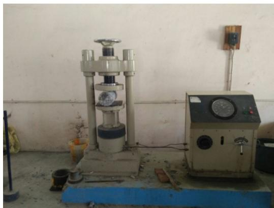
**Figure 8** Testing machine
