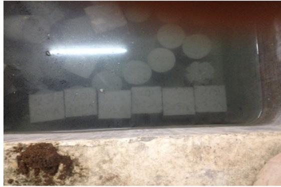
**Figure 7** Curing of cubes and cylinders
