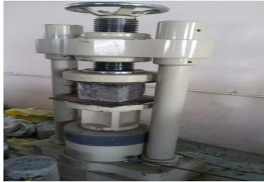
**Figure 9** Testing of cubes
