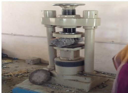
**Figure 10** Testing of cylinder
