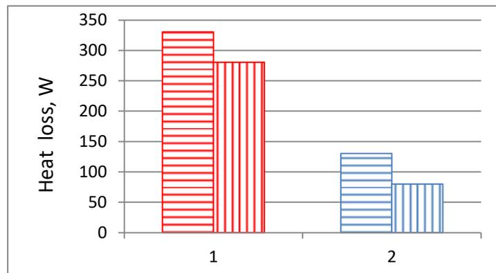
**Figure 8** Heat loss into sub-soil mass in cold period (1) warm period (2), horizontal hatching – according to method of Teploelectroproect Institute, vertical hatching – by V.D. Machinsky's method
