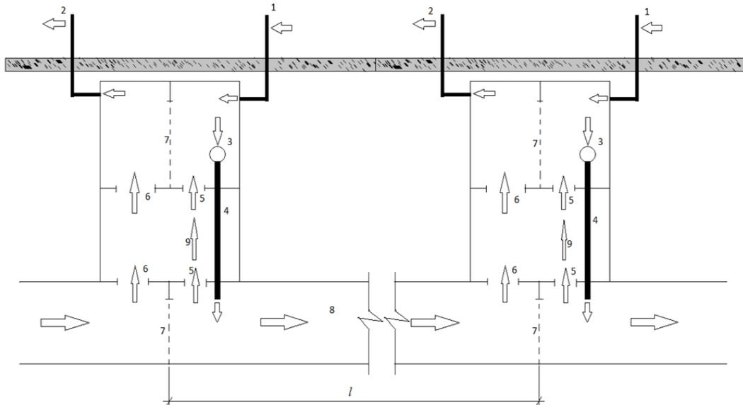
**Figure 1** The scheme of an underground tunnel, where 1 – inlet duct, 2 – exhaust duct, 3 - fan, 4 - air duct, 5 – openings for natural ventilation with a ladder for the service staff, 6 – technological aperture for service staff, 7 - door, 8 – collector, collector site  $l$ -length, 9 – recirculation contour.
