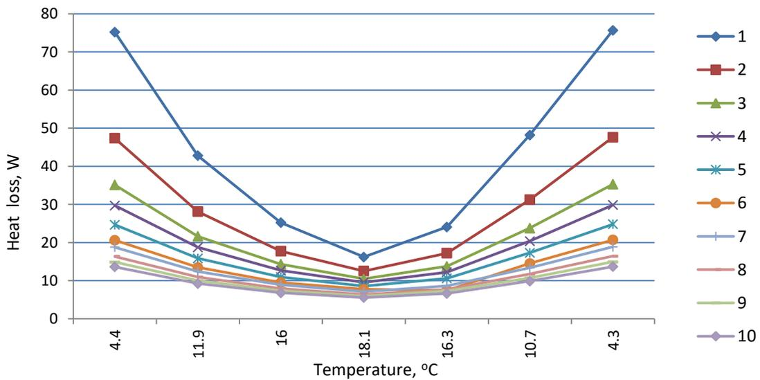
**Figure 5** Variation of heat loss parameter for underground tunnel into sub-soil during warm period depending on outdoor air temperature. On axis X average temperatures of external air for the city of Moscow in months April, May, June, July, August, September, October are postponed. Schedules 1-8 show as thermal losses would change if the tunnel would be located at a depth from 1 m to 8 m, with growth of depth by 1 m.
