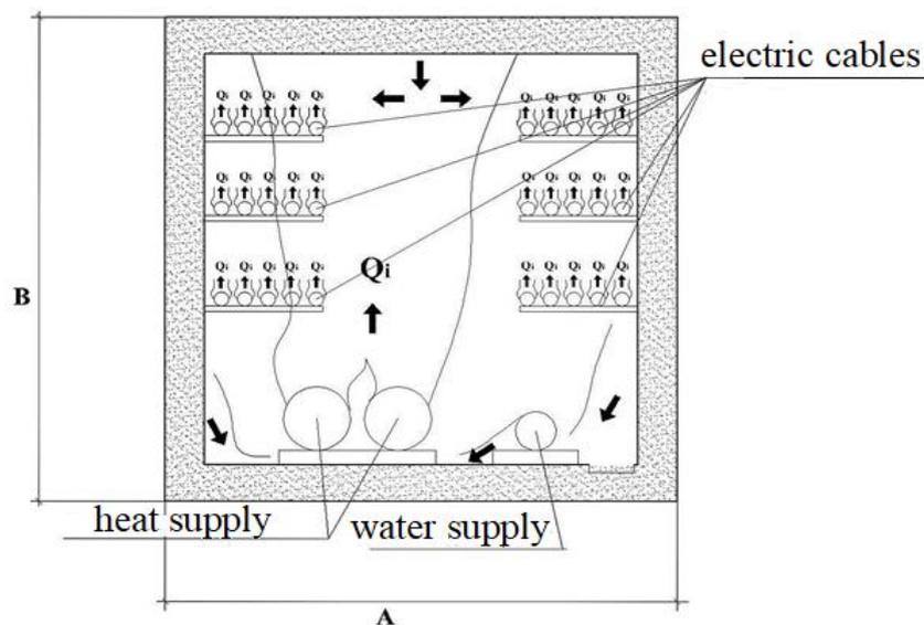
**Figure 2** The scheme of an arrangement of communications in a tunnel. Q - thermal streams from heat supply and electric cables, A и B - the tunnel sizes.
