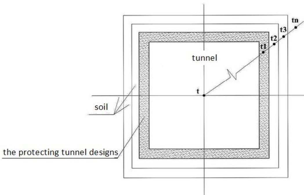
**Figure 3** Scheme of cross section of a tunnel. t - air temperature in a tunnel, t<sub>1</sub>, t<sub>2</sub>, t<sub>3</sub>, t<sub>n</sub> - temperatures of layers of earth surrounding a tunnel.
