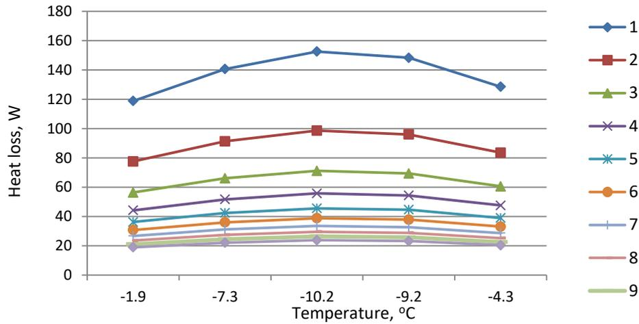
**Figure 4** Variation of heat loss parameter for underground tunnel into sub-soil during cold period depending on outdoor air temperature. On axis X average temperatures of external air for the city of Moscow in months November, December, January, February and March are postponed. Schedules 1-8 show how thermal losses would change if the tunnel would be located at a depth from 1 m to 8 m, with growth of depth by 1 m.
