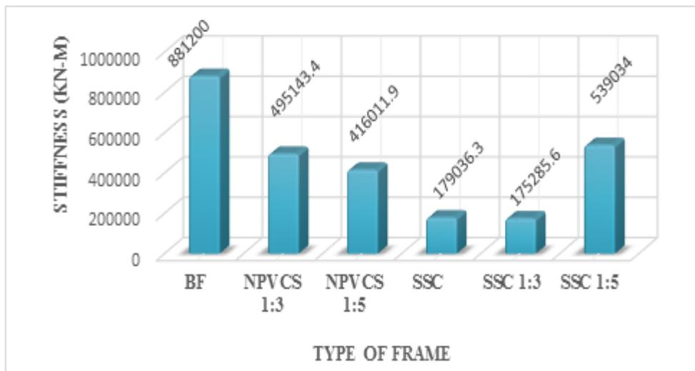
**Figure 4** Stiffness for various frames
