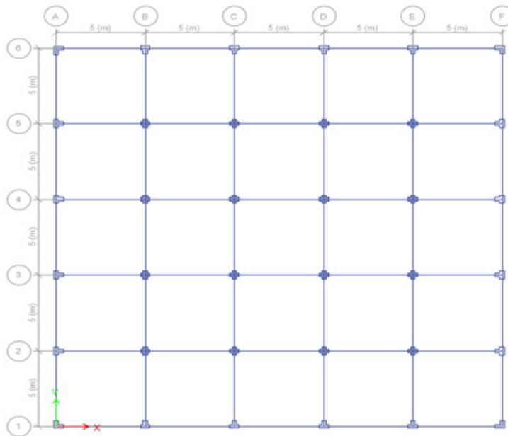
Figure 3 Plan with L, Cross & T- shaped columns
