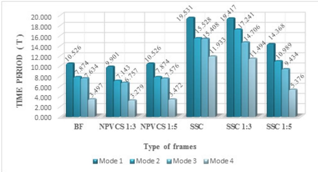
**Figure 3** Time periods for frames with special shaped beams and columns
