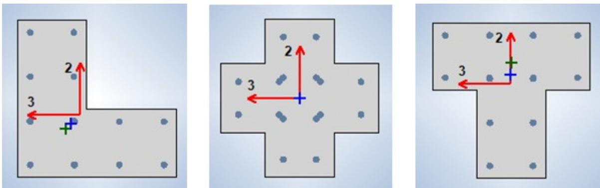
Figure 1 L, Cross & T shaped column's cross sections
