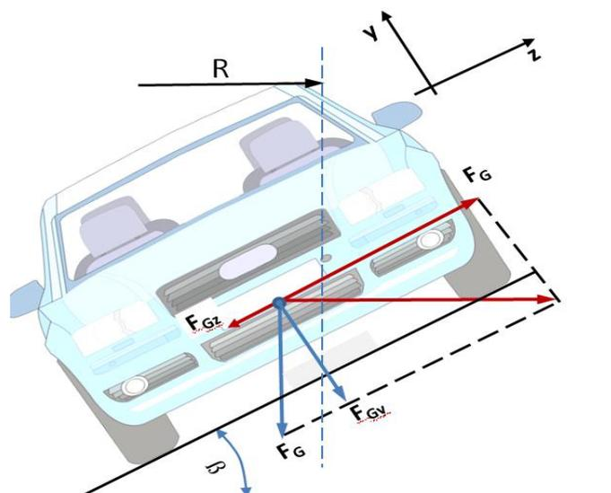
**Figure 1** Forces which influence on the vehicle during movement in curve with lateral slope
