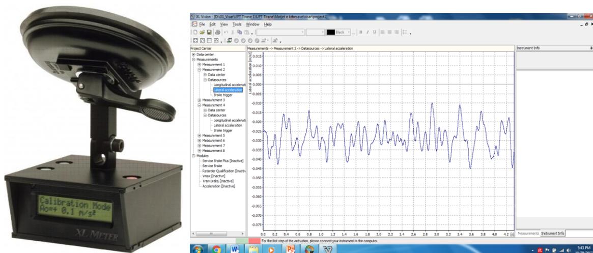
Figure 5 XL Meter Pro device for measurement of lateral acceleration with XL Vision software
