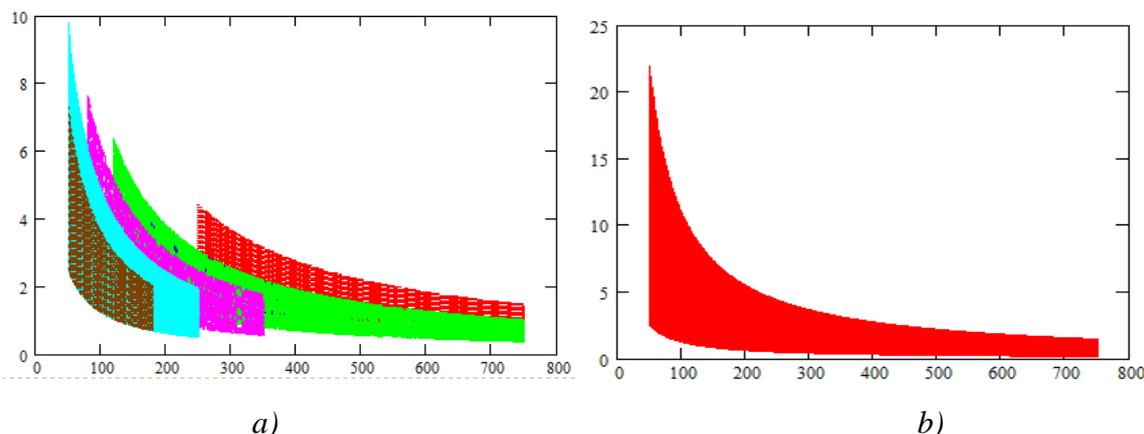
**Figure 2** Margins of lateral acceleration: a) as per road category b) full range of values R and v
