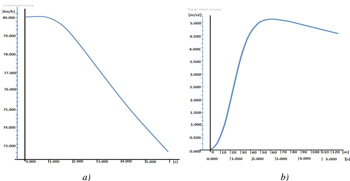
**Figure 4** Relation between lateral acceleration and changes of vehicle velocity (80km/h)
