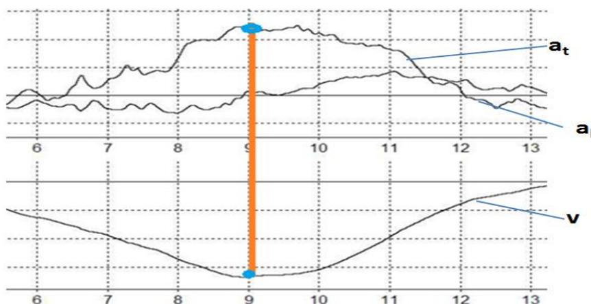
Figure 6 Measured lateral acceleration and changes of velocity of vehicle in curve
