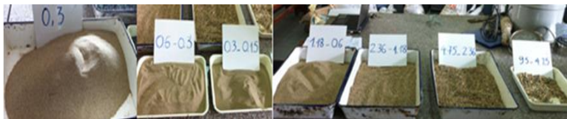
Figure 3 Particle size of sand after sieved according to ASTM C136-01 [2]
